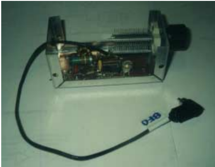
The Beat Frequency Oscillator (BFO) module.
