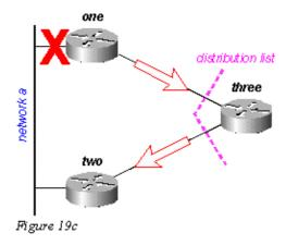
Router Two replies that Network A is reachable; Router Three now has a valid route:
