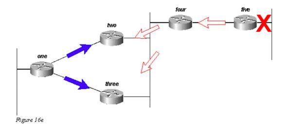
Routers Two and Three reply to the query from Router Four; Routers Two and Three are now passive for 192.168.3.0/24:
