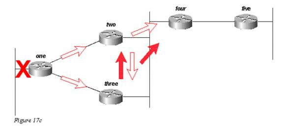
Router Four, when it receives the queries from Routers Two and Three, replies that 10.1.1.0/24 is unreachable (note that Router Four has no knowledge of the subnet in question, since it only has the 10.0.0.0/8 route):
