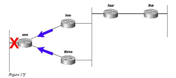
The query, in this case, is bounded by the autosummarization at Routers Two and Three. Router Five does not participate in the query process, and is not involved in the re–convergence of the network. Queries can also be bound by manual summarization, autonomous system borders, and distribution lists.
