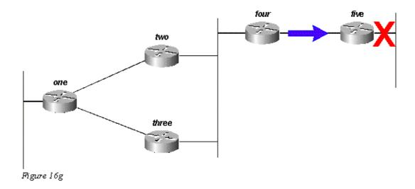
It is important to understand that although there may be other query paths or processing orders, all routers in the network process a query for network 192.168.3.0/24 when that link goes down. Some routers may end up processing more than one query (Router One in this example). In fact, if the queries were to reach the routers in a different order, some would end up processing three or four queries. This is a good example of an unbounded query in an EIGRP network.
