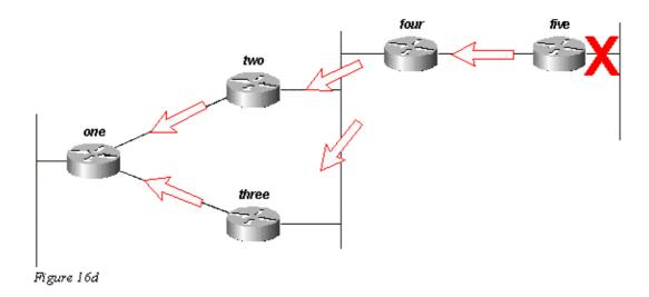
Router One replies to both queries with unreachables; Router One is now passive for 192.168.3.0/24:
