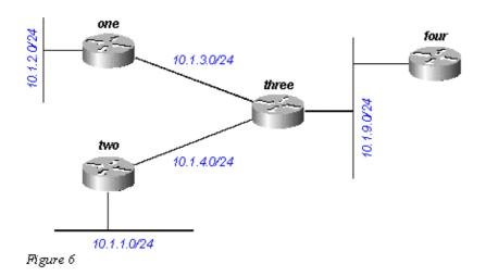
Router Three receives a query concerning 10.1.2.0/24 (which it reaches through Router One) from Router Four. If Three does not have a successor for this destination because a link flap or other temporary network
