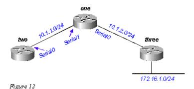
Router One has a static route to the network 172.16.1.0/24 configured through interface Serial 0:
