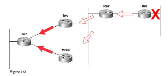
For simplicity, let us assume that Router One receives the query from Router Three first, and marks the route as unreachable. Router One then receives the query from Router Two. Although another order is possible, they will all have the same final result.
