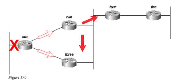
Router Three, when it receives the query from Router One, marks the destination as unreachable and queries Routers Two and Four:
