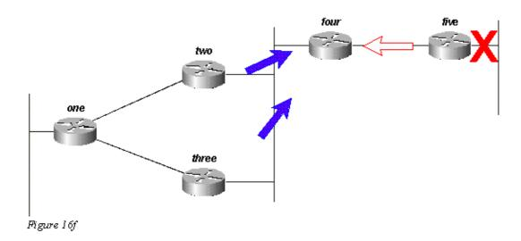
Router Five, upon receiving the reply from Router Four, removes network 192.168.3.0/24 from its routing table; Router Five is now passive for network 192.168.3.0/24. Router Five sends updates back to Router Four so the route is removed from the topology and routing tables of the remaining routers.
