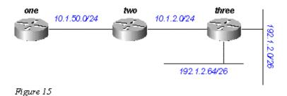
Router Three is injecting external routes to 192.1.2.0/26 and 192.1.2.64/26 into EIGRP using the **redistribute connected** command, as shown in the configurations below.
