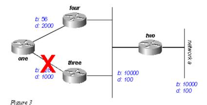
Router One sees that it has two routes to Network A: one through Router Three and another through Router Four.
