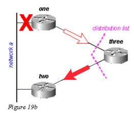
Router Two examines its topology table and finds that it has a valid connection to Network A. Note the query was not affected by the distribution list in Router Three:
