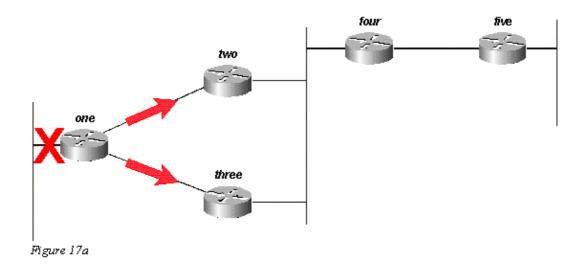
Router Two, on receiving the query from Router One, marks the route as unreachable (because the query is from its successor) and then queries Routers Four and Three:
