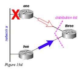
Router Three builds the reply to the query from Router One, but the distribution list causes Router Three to send a reply that Network A is unreachable, even though Router Three has a valid route to Network A:
