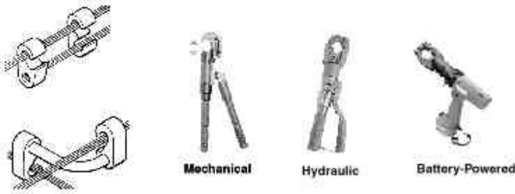
FIGURE 23-50 HIGH-COMPRESSION CONNECTORS AND TYPICAL CRIMPING TOOLS
