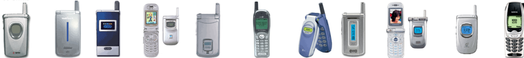
SAMSUNG SCH-X580 72 GRAMS SK TELETECH IM-5100 88 GRAMS LG VX1 108 GRAMS TOSHIBA A20131 105 GRAMS LG 4NE1 106 GRAMS SANYO SCP-6200 75 GRAMS CASIO A2012CA 106 GRAMS KYOCERA A1012K 93 GRAMS SANYO A3011SA 97 GRAMS SYNERTEK S-200 120 GRAMS SAMSUNG SCH-X290 89 GRAMS
