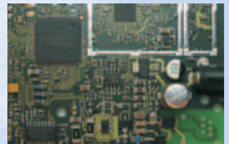
An example of a final PCB for 2.4 GHz, where the RF form factor can be as small as 400 mm 2
