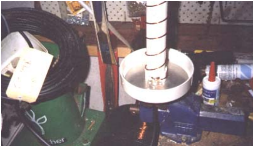
Daryl Clarkson in New Zealand made these aerials below pretty much verbatim to what I described. He's gone ape and made 15 and 22 turn versions as well! He reckons they work very well on a 3.7Km link he's using. The final picture is the aerial mounted and in use!
