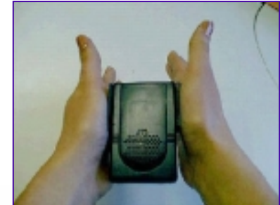
Electrocardiogra m monitor that transmits patient data over a regular telephone line
