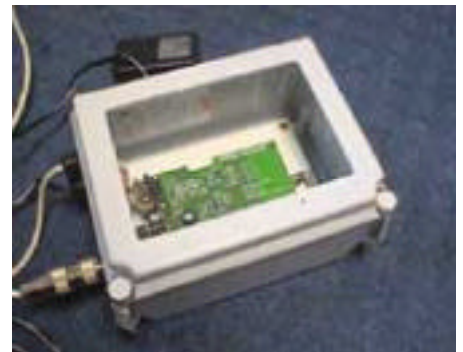
World Wireless Communications 900 SS 56kpbs low cost radio, in field protection case.
