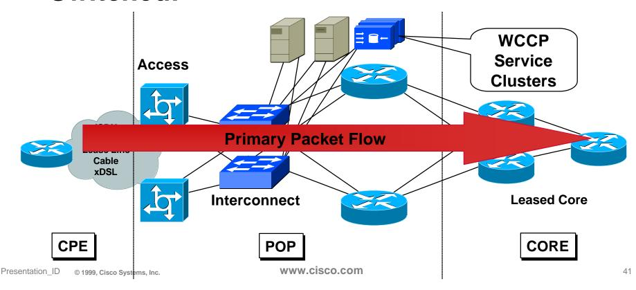
Work with the multi-level L2/L3 redundancy of the ISP POP. Equal paths in the IGP + CEF leads packet asymmetry.
