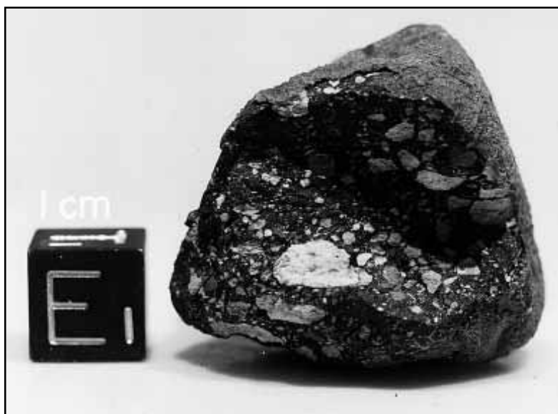
Lunar meteorite ALHA81005. This 31 g (ping pong ball-sized) meteorite is a breccia rich in light colored anorthosite fragments melted and mixed together by impacts in the lunar highlands. Other lunar meteorites are dark colored basalts from the mare. The scale is 1 cm across.
