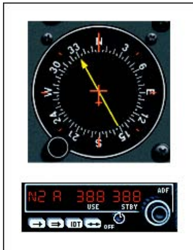
Figure 7-2. ADF indicator instrument and receiver.
