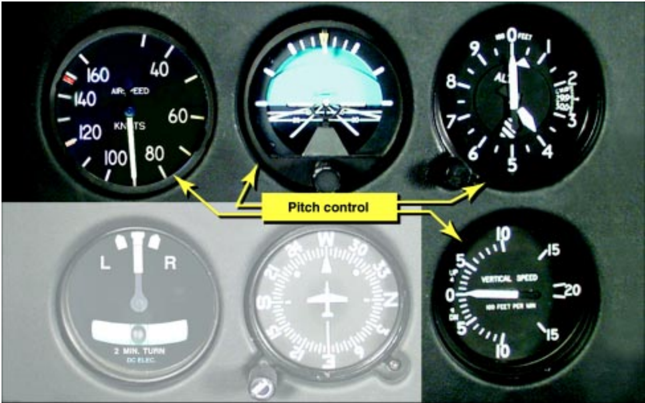
Figure 6-2. The flight instruments for pitch control are the airspeed indicator, attitude indicator, altimeter, and vertical speed indicator.
