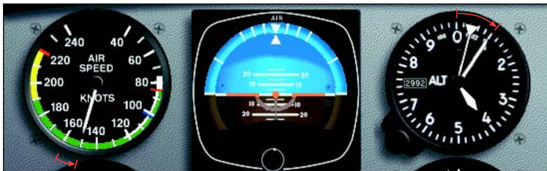
Figure 5-20. Airspeed low and altitude high (lower pitch).
