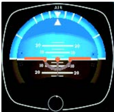
Figure 5-4. Pitch correction for level flight, half-bar width.
