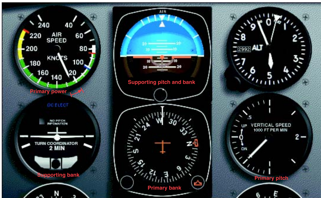
Figure 5-30. Constant airspeed descent, airspeed high—reduce power.
