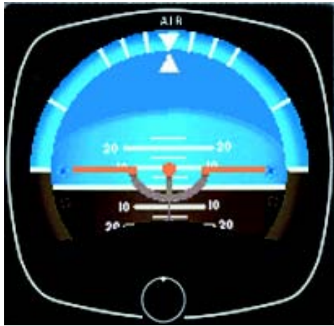
Figure 3-29. The dial of this attitude indicator has reference lines to show pitch and roll.
