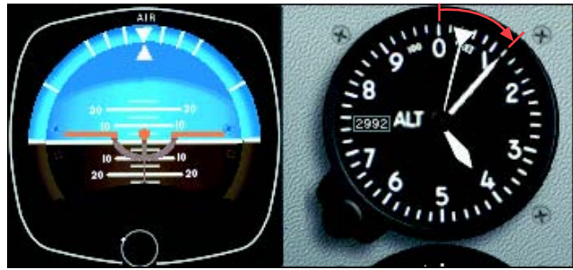
Figure 5-7. Using the altimeter for pitch interpretation, a high altitude means a nose-high pitch attitude.
