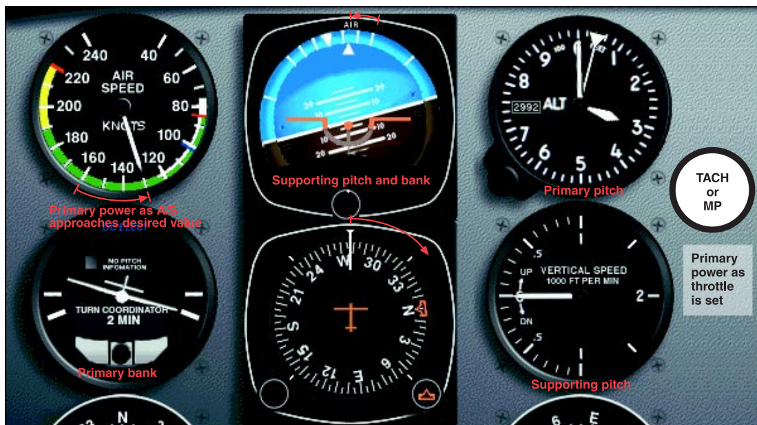
Figure 5-38. Change of airspeed in turn.
