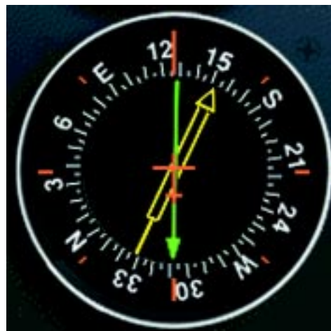
Figure 3-25. The compass card in this RMI is driven by signals from a flux valve and it indicates the heading of the aircraft opposite the upper center index mark.
