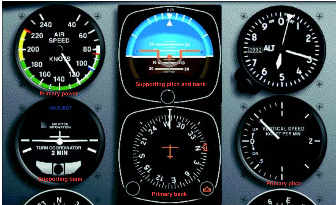
Figure 5-27. Stabilized climb at constant rate.
