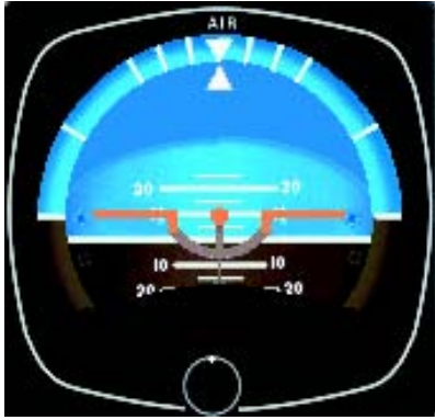
Figure 5-6. Pitch correction for level flight, three-bar width.
