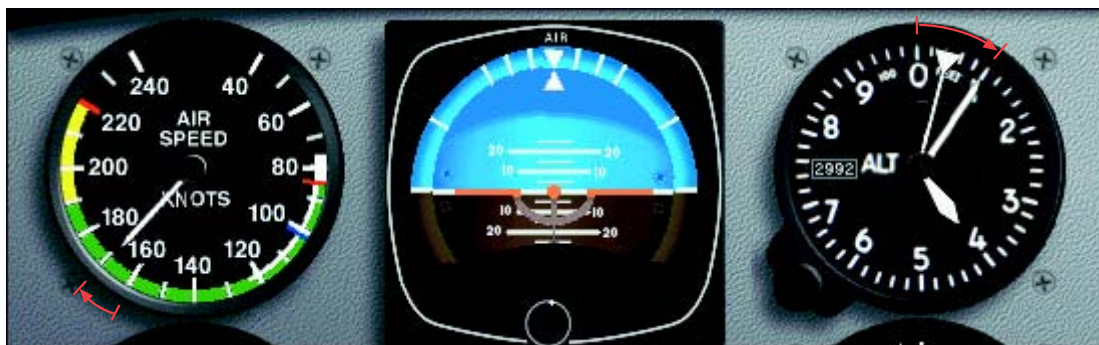
Figure 5-21. Airspeed and altitude high (lower pitch and reduce power).
