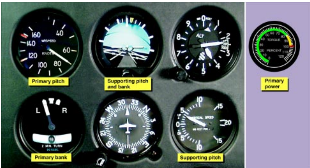
Figure 6-12. Flight instrument indications for a stabilized left climbing turn at a constant airspeed.
