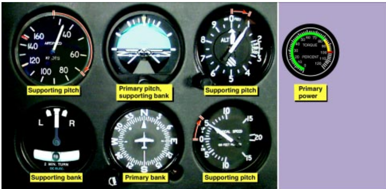
Figure 6-13. Flight instrument indications during an instrument takeoff.
