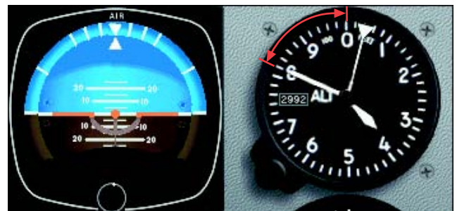
Figure 5-11. Altitude error, greater than 100 feet.
