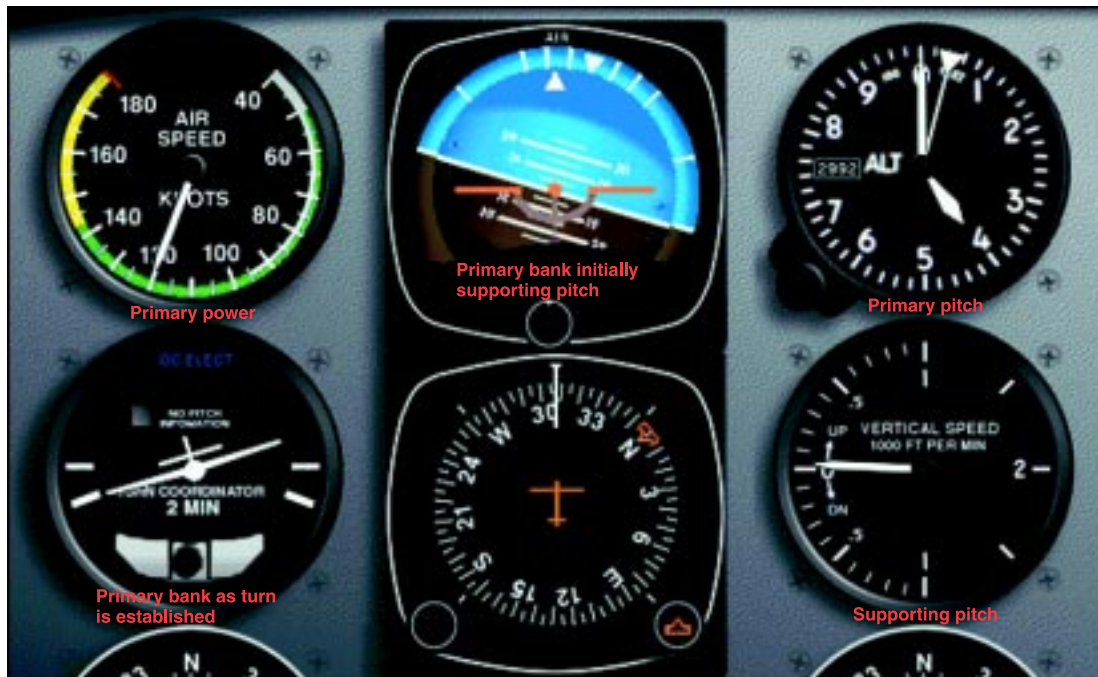
Figure 5-33. Standard-rate turn, constant airspeed.
