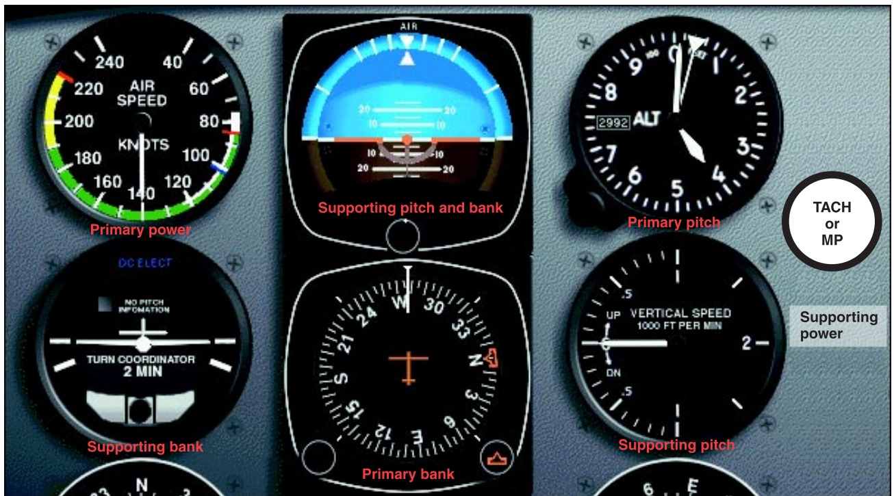
Figure 5-22. Straight-and-level flight (normal cruising speed).
