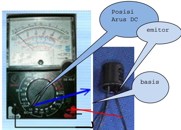
Gambar 2-68. Pengukuran arus bocor transistor NPN
