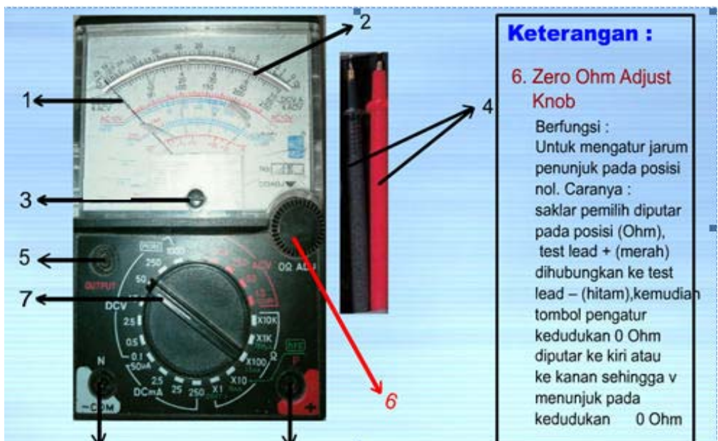
Gambar 2-40. Fungsi Ohm adjust knob
