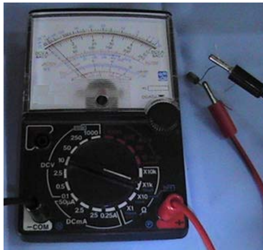
Gambar 2-84. Pengetesan basis kolektor reverse
