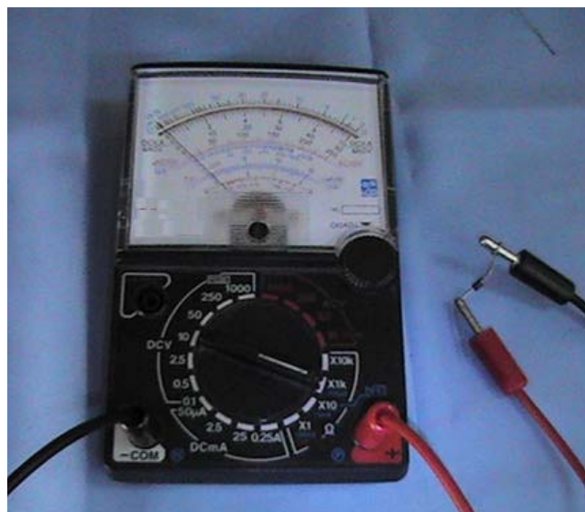
Gambar 2-78. Pengetesan dioda bias balik
