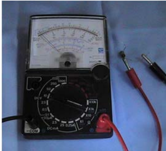
Gambar 2-83. Pengetesan basis emitor reverse
