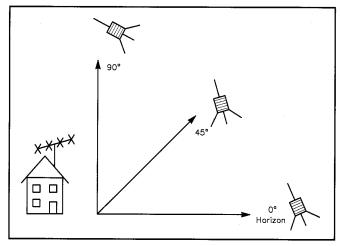
Fig 1—*Elevation* describes the vertical position of the satellite in the sky relative to your station. It's expressed as degrees from  $0^{\circ}$  to 90°. An elevation of 0° is right at your horizon. A 90° elevation is directly overhead.
