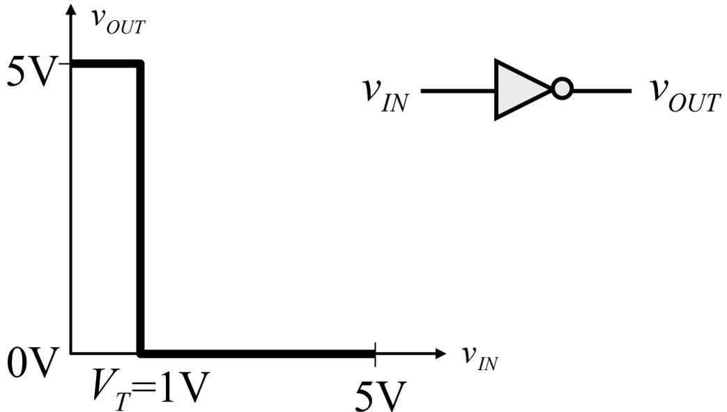
The T1000 model laptop desires gates that satisfy the static discipline with voltage thresholds. Does our inverter qualify?
