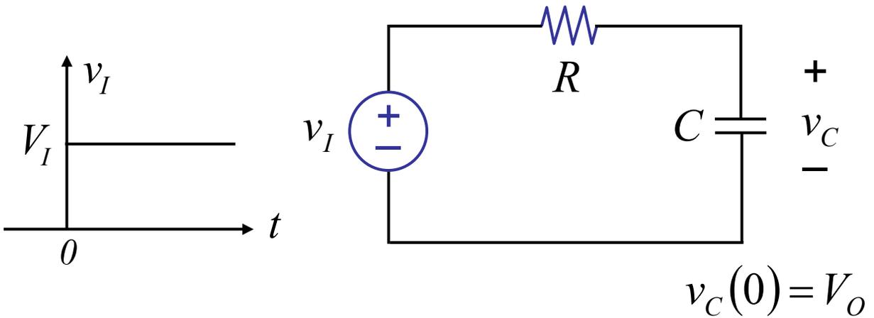
$$v_C = V_I + (V_O - V_I) e^{\frac{-t}{RC}} \quad \text{—————} \quad \textcircled{1}$$
