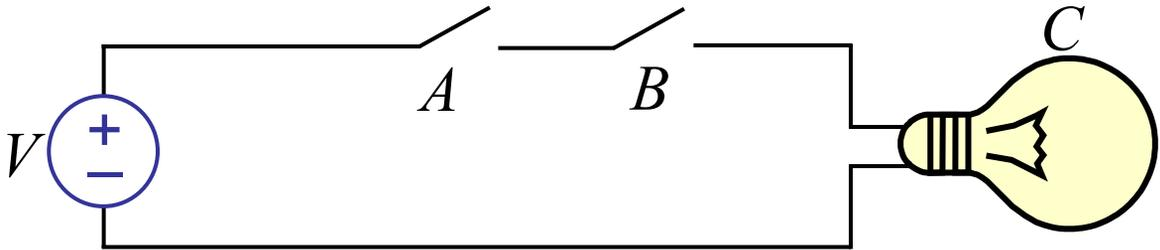
Bulb  $C$  is ON if  $A$  AND  $B$  are ON,
