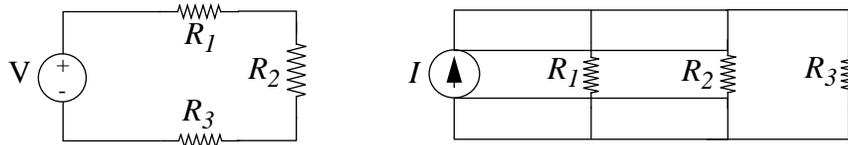
**Exercise 1-2:** Beginning with 1k resistors, synthesize a resistor of 3/5k and a resistor of 5/3k. Use no more than four 1k resistors in each case.
