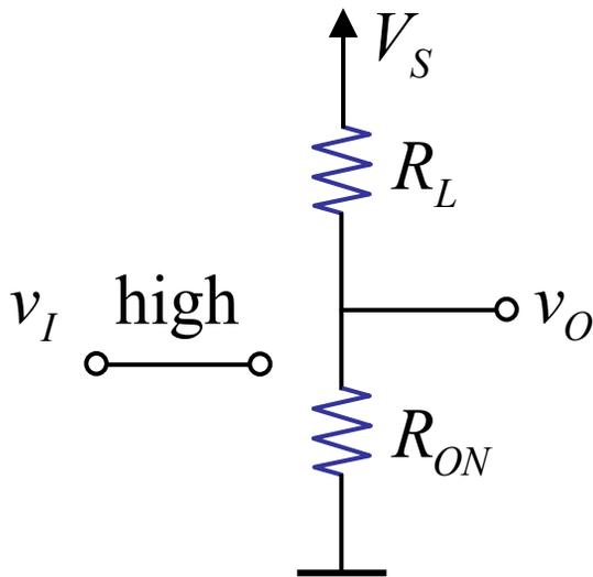
$$P = \frac{V_S^2}{R_L + R_{ON}}$$
