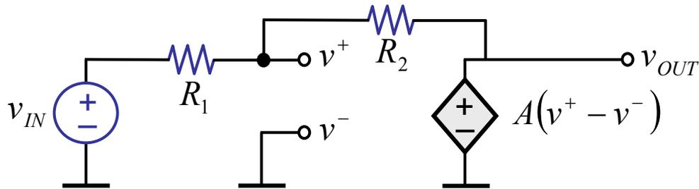
$$v_{OUT} = A(v^+ - v^-)$$
