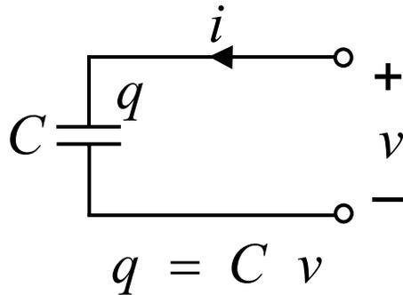
$$\begin{aligned} i &= \frac{dq}{dt} \\ &= \frac{d(Cv)}{dt} \\ &= C \frac{dv}{dt} \end{aligned}$$
