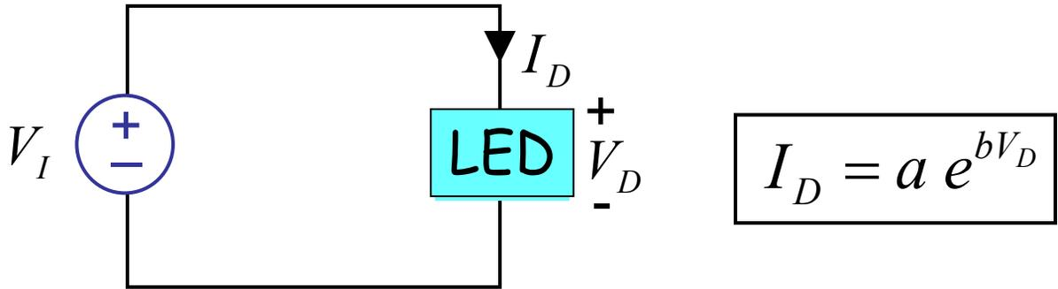
Small signal response:  $i_d = I_D b v_d$
