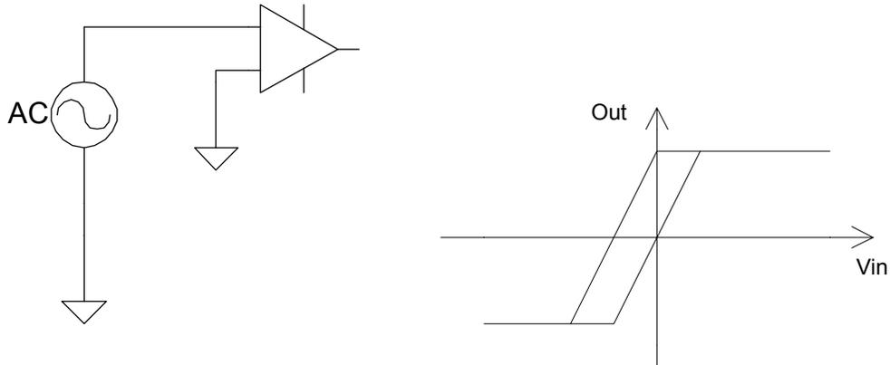
The hysteresis varies with temperature which can be changed with a can of liquid cold or a hot air gun.
