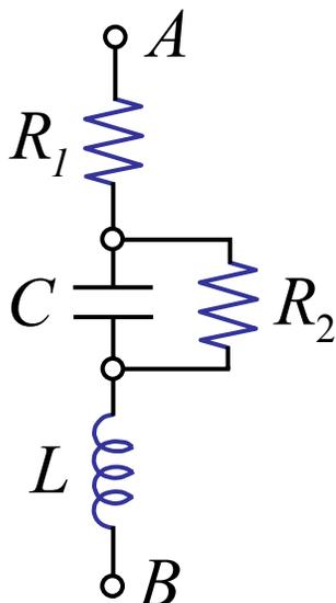
$$\begin{aligned} Z_{AB} &= R_1 + Z_C \parallel R_2 + Z_L \\ &= R_1 + \frac{Z_C R_2}{Z_C + R_2} + Z_L \\ &= R_1 + \frac{R_2}{1 + j\omega C R_2} + j\omega L \end{aligned}$$
