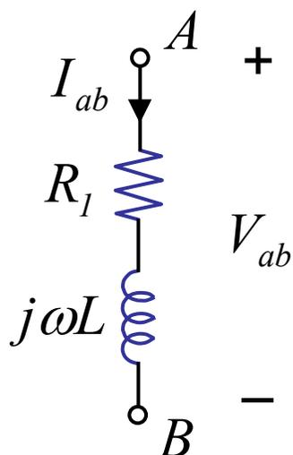
$$Z_{AB} = \frac{V_{ab}}{I_{ab}} = R_1 + j\omega L$$
