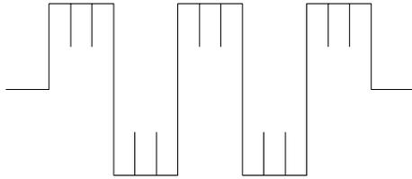
Part 4: Place feedback around Schmitt trigger and add a capacitor to create triangle and square waves.
