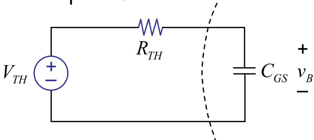
$$R_{TH} = R_L \parallel R_{ON}$$
