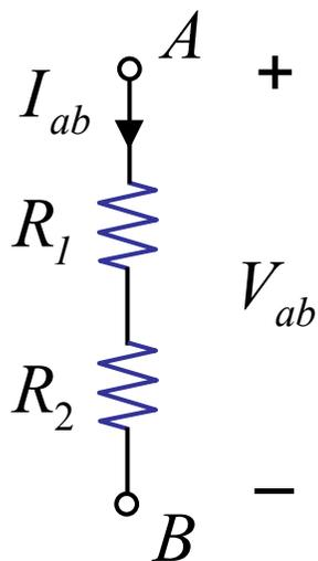
$$R_{AB} = \frac{V_{ab}}{I_{ab}} = R_1 + R_2$$
