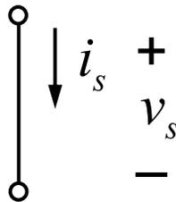
$$v_s = \left. \frac{\partial V_S}{\partial i_S} \right|_{i_S = I_S} \cdot i_s$$
