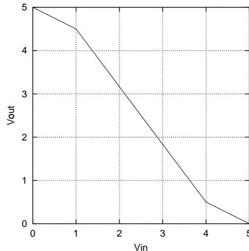
For suitable choices of the voltages  $V_{OL}$ ,  $V_{IL}$ ,  $V_{IH}$ , and  $V_{OH}$  this inverter obeys the static discipline (see Figure 5.8 on page 250 in the textbook).
