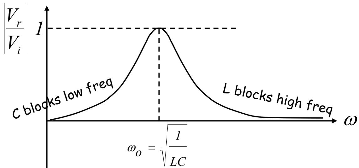
$$\begin{aligned}\frac{V_r}{V_i} &= \frac{R}{j\omega L + \frac{1}{j\omega C} + R} \\ &= \frac{j\omega RC}{1 - \omega^2 LC + j\omega RC}\end{aligned}$$
