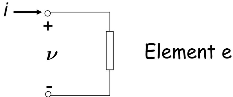
Current is taken to be positive going into the positive voltage terminal
