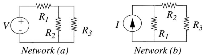
**Exercise 2.3:** Following the node method, develop a set of simultaneous equations for the network shown below that can be used to solve for the three unknown node voltages in the corresponding network. Express these equations in the form
