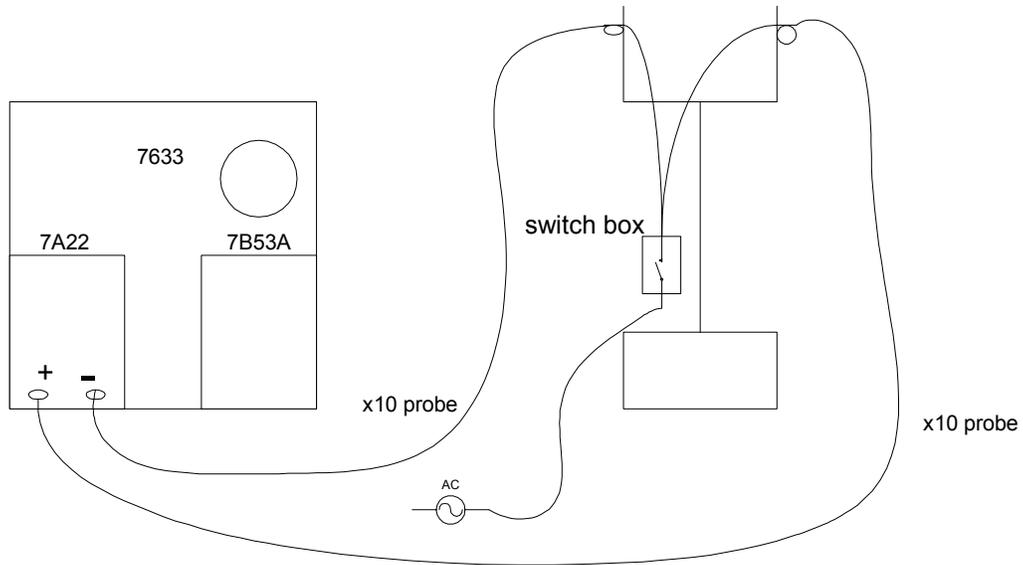
We use (2) X10 probes on differential amplifier 7A22 and using caution not to ground any points and the amplifier plug in should be set on AC not DC coupling set the voltage to 5 volts range.
