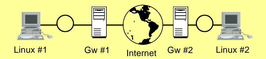
If Linux #1 needs a connection to Linux #2, attackers can sniff packets on the Internet, on LAN #1, on LAN #2 or on either gateway.
