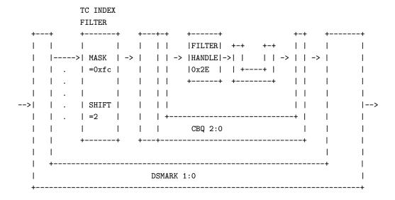
The packet arrives, then, set with 0xb8 value at DS field. As we explained before, dsmark qdisc identified by 1:0 id in the example, retrieves DS field and store it in skb->tc\_index variable. Next step in the example will correspond to the filter associated to this qdisc (second line in the example). This will perform next operations:
