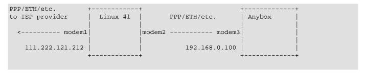
In the above drawing, a Linux box with IP\_MASQUERADING is installed as Linux #1 and is connected to the Internet via PPP, Ethernet, etc. It has an assigned public IP address of 111.222.121.212. It also has another network interface (e.g. modem2) connected to allow incoming network traffic be it from a PPP connection, Ethernet connection, etc.
