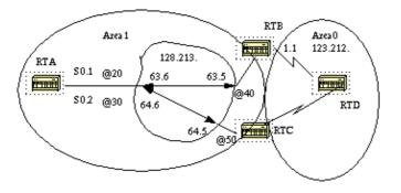
In the above diagram, on RTA, we can split Serial 0 into two point-to-point subinterfaces, S0.1 and S0.2. This way, OSPF will consider the cloud as a set of point-to-point links rather than one multi-access network. The only drawback for the point-to-point is that each segment will belong to a different subnet. This might not be acceptable since some administrators have already assigned one IP subnet for the whole cloud.
