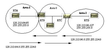
In the above diagram, RTB is summarizing the range of subnets from 128.213.64.0 to 128.213.95.0 into one range: 128.213.64.0 255.255.224.0. This is achieved by masking the first three left most bits of 64 using a mask of 255.255.224.0. In the same way, RTC is generating the summary address 128.213.96.0 255.255.224.0 into the backbone. Note that this summarization was successful because we have two distinct ranges of subnets, 64–95 and 96–127.
