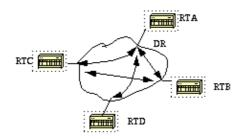
In the above diagram, it is essential for RTA's interface to the cloud to be elected DR. This is because RTA is the only router that has full connectivity to other routers. The election of the DR could be influenced by setting the ospf priority on the interfaces. Routers that do not need to become DRs or BDRs will have a priority of 0 other routers could have a lower priority.
