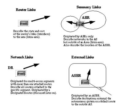
As indicated above, the router links are an indication of the state of the interfaces on a router belonging to a certain area. Each router will generate a router link for all of its interfaces. Summary links are generated by ABRs; this is how network reachability information is disseminated between areas. Normally, all information
