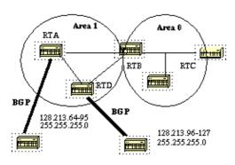
In the above diagram, RTA and RTD are injecting external routes into OSPF by redistribution. RTA is injecting subnets in the range 128.213.64–95 and RTD is injecting subnets in the range 128.213.96–127. In order to summarize the subnets into one range on each router we can do the following:
