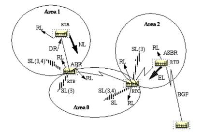
Link-state advertisements are broken into five types. Router Links (RL) are generated by all routers. These links describe the state of the router interfaces inside a particular area. These links are only flooded inside the
