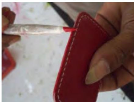
Gambar 3.21. Finishing pengecatan cat tepi
