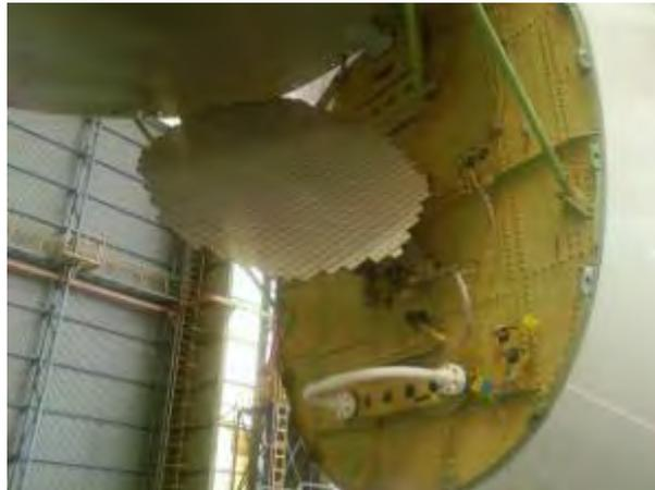
Antena *glideslope* diatas antenna radar, antenna *localizer* dibawah antenna radar
