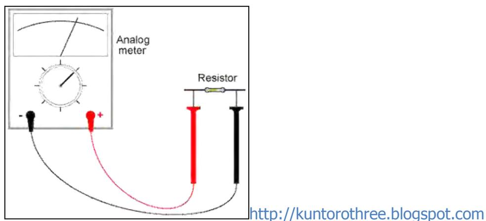
Gambar 9 . Mengukur Tahanan (*Resistance*)
