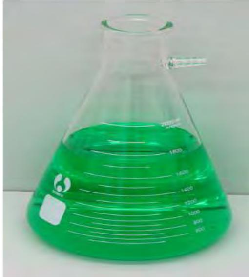
**Gambar 11. Filtering flask**
