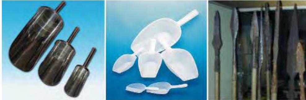
**Gambar 65. Hand scoop (atas), Plastic scoop (bawah) DAN Tombak pengambil sampel (spear)**
