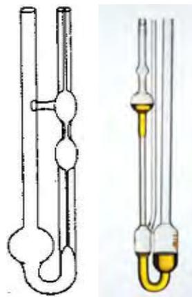
Gambar 25. Viskosimeter "Ubbelohde"
