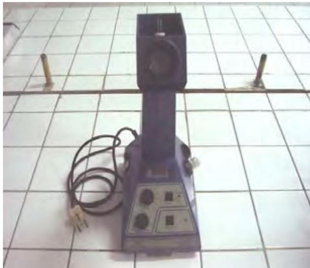
Gambar 29. Alat "Melting Point Aparatus"
